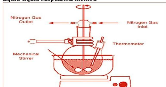
**Fig 3. Method of quasi-emulsion solvent diffusion**
